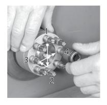
Step 2: Now tighten these 4 jackbolts crosswise with 50% of the recommended jackbolt torque.
